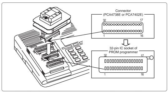
Figure 3.3 Attaching the adapter to a PROM programmer (PCA4738E or PCA7402E)
